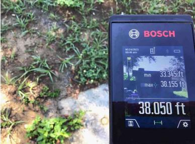
Distance measured from septic tank cover to well inside shed does not meet minimum distance requirements.
